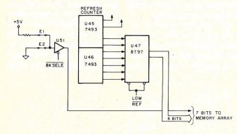
Fig. 4. Address path during refreshing.
